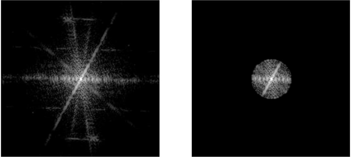
Fig. 2. Appearing of blur and ringing effect after high frequency information cut off for  $p = 4$ .
