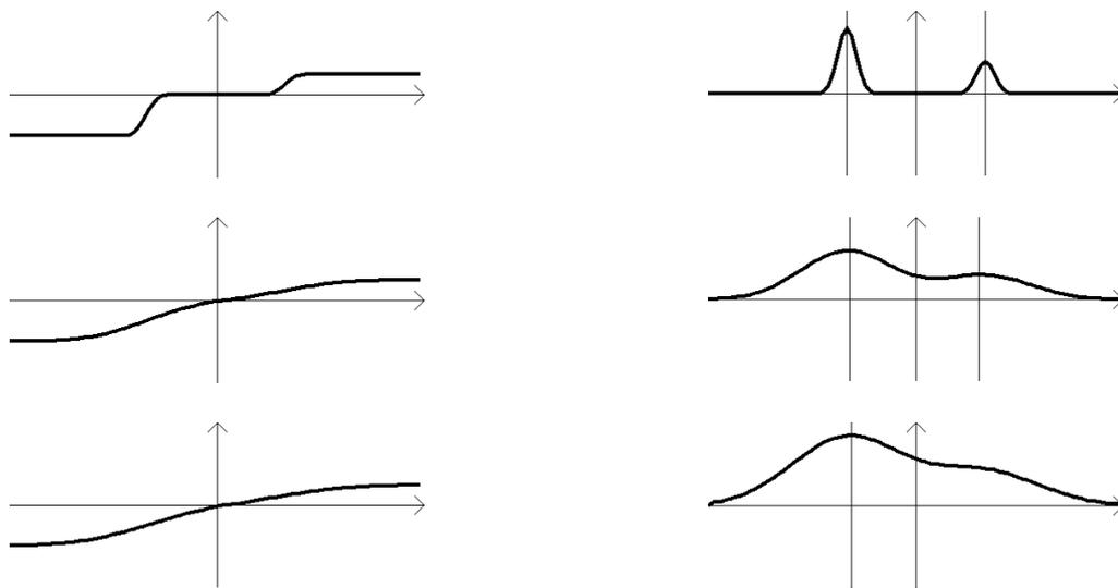
Fig. 4. The effects of edge masking and edge displacement for image blurring. Left: original edge profiles; right: gradient values with marked local maxima. Top row: low blur; middle: medium blur; bottom: strong blur.
