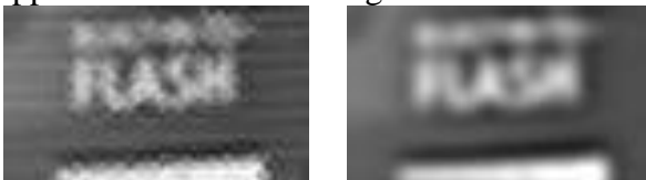
a) The proposed super-resolution method (6) b) Super-resolution for unstable data (13) Fig. 2. Super-resolution results for 4 input images and factor s=4 for inaccurately defined warping operator.
