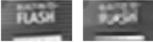
c) The proposed super-resolution method (6) e) Regularization-based image interpolation [11] Fig. 1. Super-resolution results using 4 input images and scale factor s=4 .
